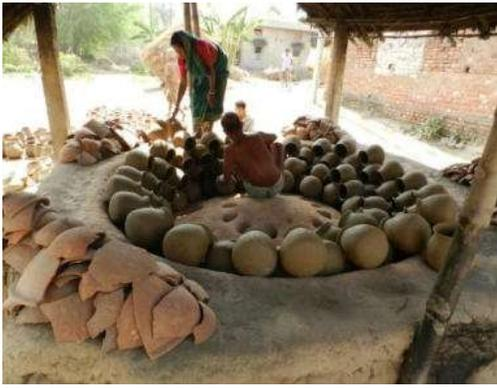
Fig.13. Arrangement of vessels on kiln
